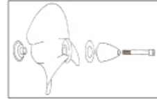
Long Hub Installation
